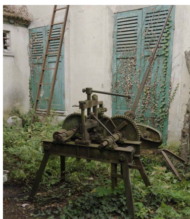
Cintreuse a bras. Phot. Philippe Ayrault IVR11_20097701534NUC4A
